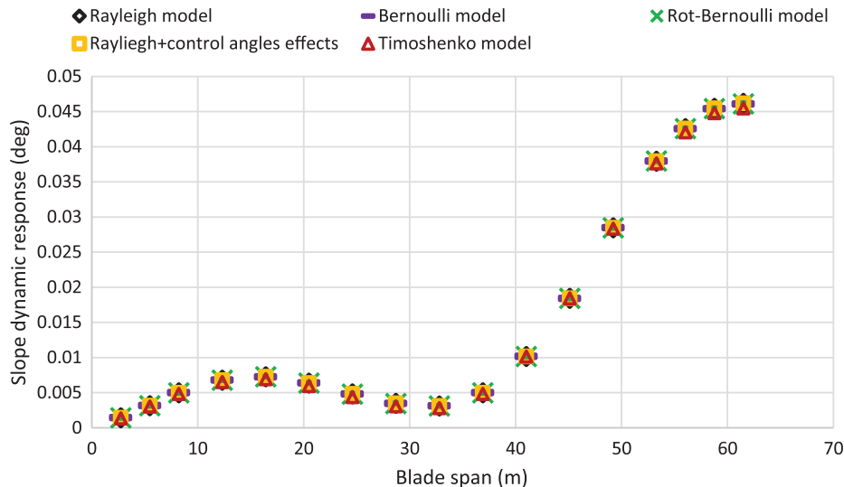
Fig. 19. Edge-wise slope distribution along the blade span.
