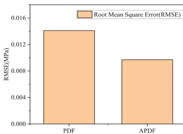
Fig. 8. Comparison of predictive performance between best-performing fixed-weight PDF and APDF.
