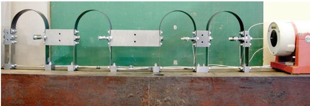
Fig. 4. A five-DoF mass-spring structure with a shaker.
