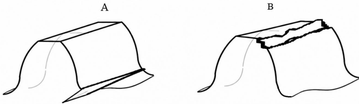
Fig 16: Crack patterns in a helical gear tooth : (A) crack, (B) spalling.
