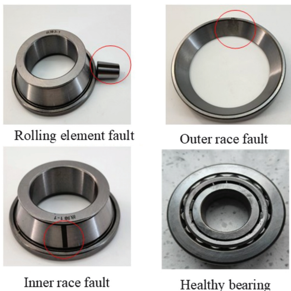
Fig. 7. Photographs of a normal bearing and typical failed bearings.
