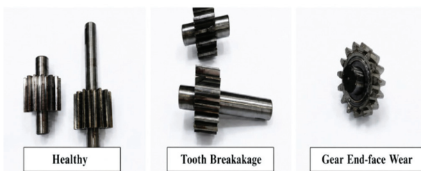
Fig. 2. Representative gear fault components
