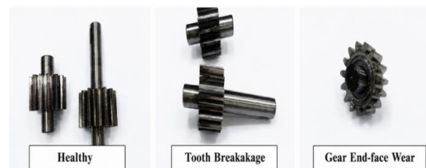
Fig. 2. Representative gear fault components
