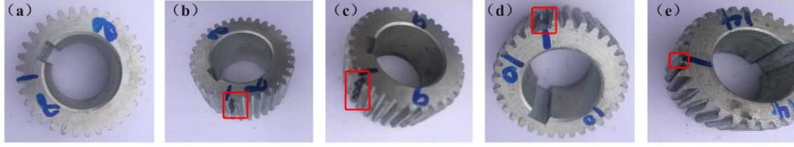
Fig. 5. Fault Details: (a) Healthy; (b) Light Pitting; (c) Medium Pitting; (d) Partial Tooth Breakage; (e) 0.3 mm × 0.5 mm Worn.
