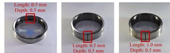
(c) Faulty bearings
