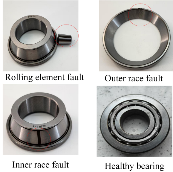
Fig. 7. Physical photographs of the normal bearing and three typical faulty bearings
