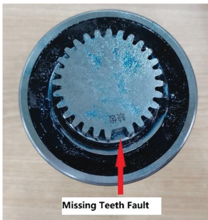
Fig. 7. A simulated missing tooth fault of the sun gear.
