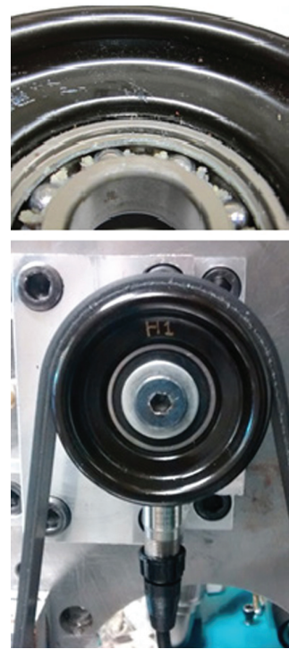
Fig. 11. Bearing with outer race fault (top) and assembled in the belt drive system (bottom).
