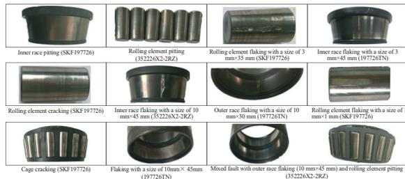
FIGURE 5. The photos of faulty bearings. These faulty bearings are naturally produced during the operation of high-speed train. The model of the experimental bearing is given in parentheses.
