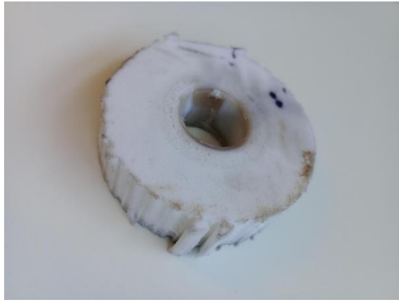
Fig. 8. Failed driving gear made of nylon using the SLS method.
