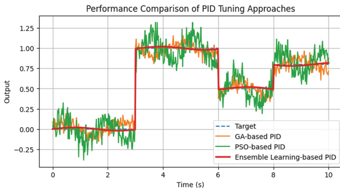
Fig. 7. GA-optimized PID, ML-assisted PSO-optimized PID, and the proposed ensemble learning-based PID controller under identical reference conditions.
